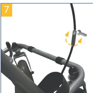
If braking is poor or too hard, the brake can be adjusted either at the brake housing above (**pic. 6**) or using the adjusting screw on the Bowden cable below (**pic. 7**) to achieve the desired braking effect.
