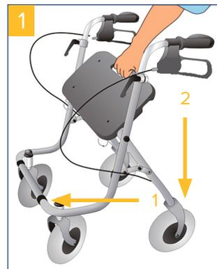
Place rollator on its wheels. Push front frame forwards by pulling the handle diagonally downwards and backwards until the rollator is standing on four wheels.
