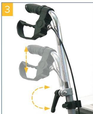
Insert push handles at least to the “**MAX**” mark in the frame tube (**pic. 3**). Secure them at the desired height by turning the locking lever clockwise. Adjust both handles to the same height.
